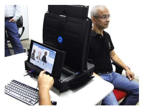
vb e-pass<sup>™</sup> portable - the integrated enrollment and verification solution used by POLITEC technicians to capture biographic and biometric data in real-time
